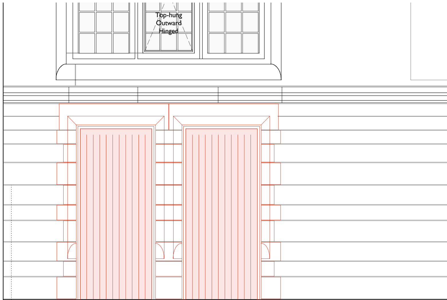
2no new oak doors, frames & lining nom overall size: 930w x 2060hmm each
